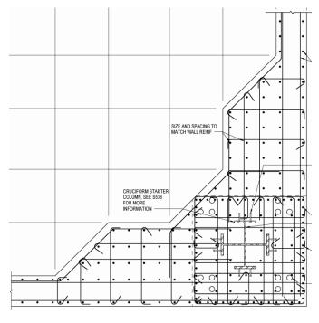
Figure 10 | Typical Mega Column (Detail 1-S332)
