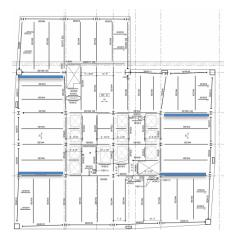
Figure 4 | Location of Composite Beams (S108)
