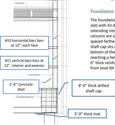
Figure 11 | Section Cut at Foundation (Detail 2-S320)
