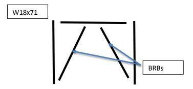
Figure 9 | Buckling Restrained Braces at Upper Levels
