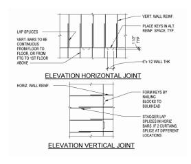
Figure 13 | Horizontal and Vertical Wall Joints (Detail 9-S304)
