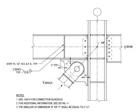
Figure 18 | Buckling Restrained Brace Pin Connection (Detail 2-S515)
