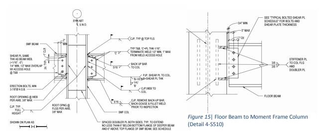
Figure 14 | Two-Sided Moment Frame Connection (Detail 1-S510)
