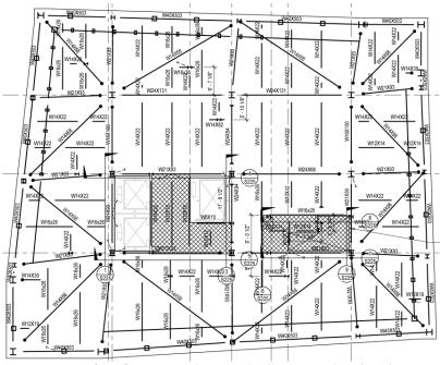
Figure 7 | Roof Framing With Diagonal Collector Members (S156)
