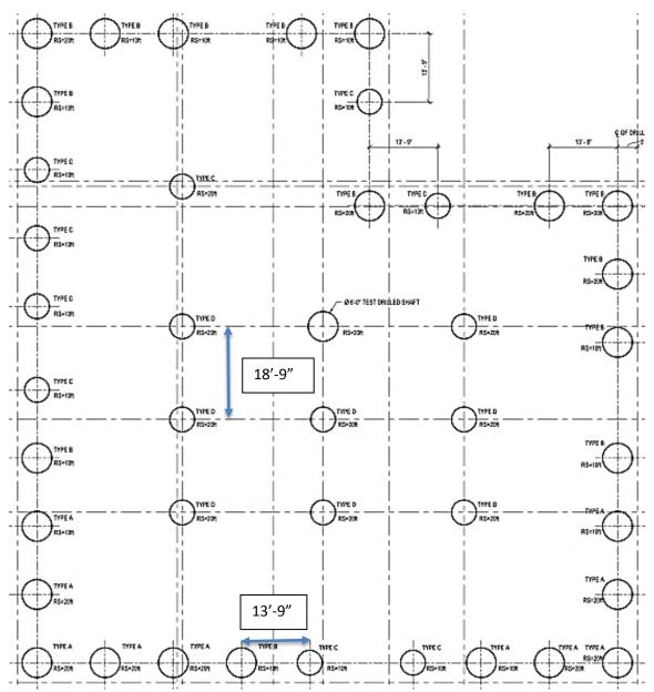
Figure 12 | Foundation Layout (S100F)
