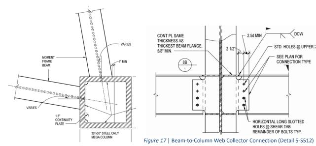
Figure 16 | Continuity Plate Through Mega Column (Detail 6-S511)
